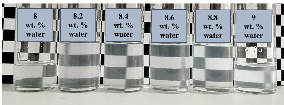
Figure F. 3. CA18-DHAc polymer solutions with different water concentrations for cloud point measurement
